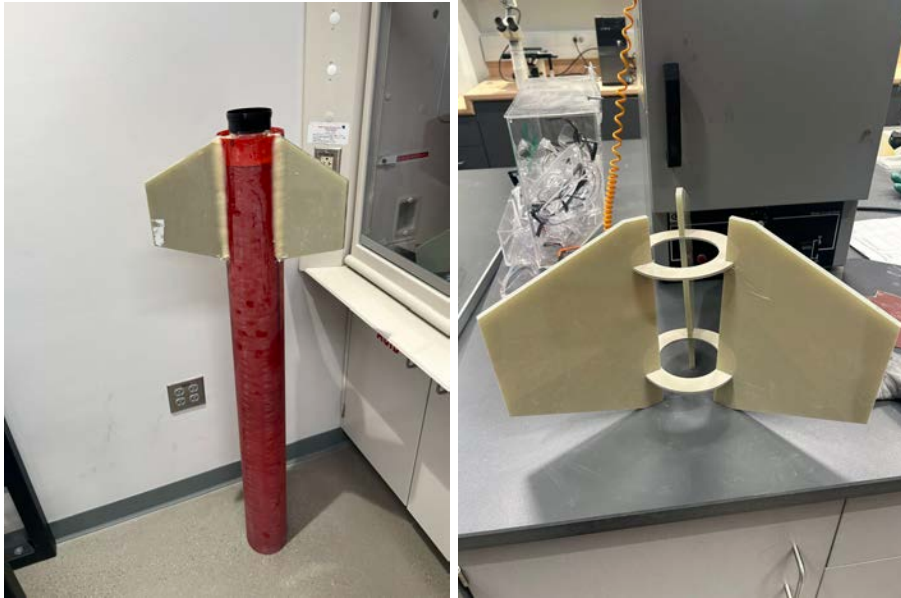
Figure 13. Motor Section Construction
