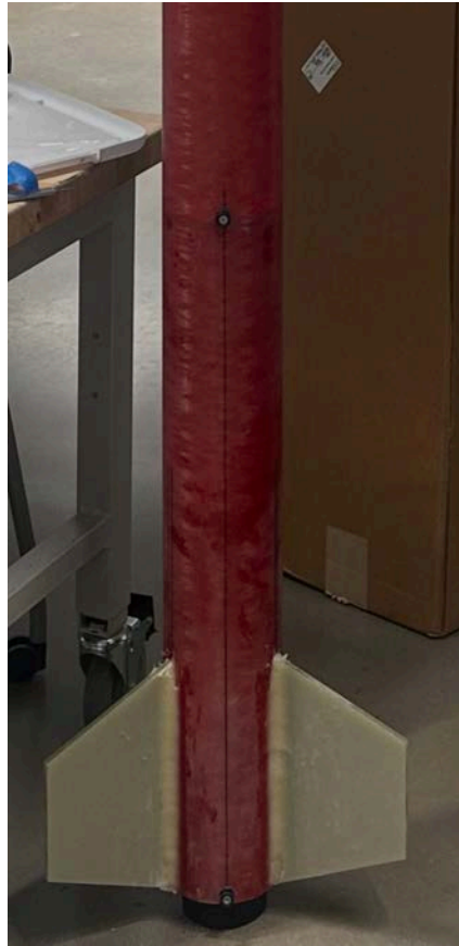
Figure 15. Location of rail buttons on rocket
