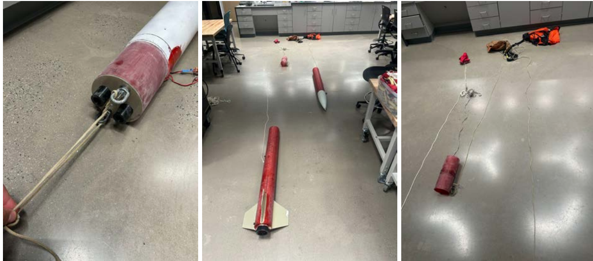
Figure 19. Layout of shock cord and rocket sections
