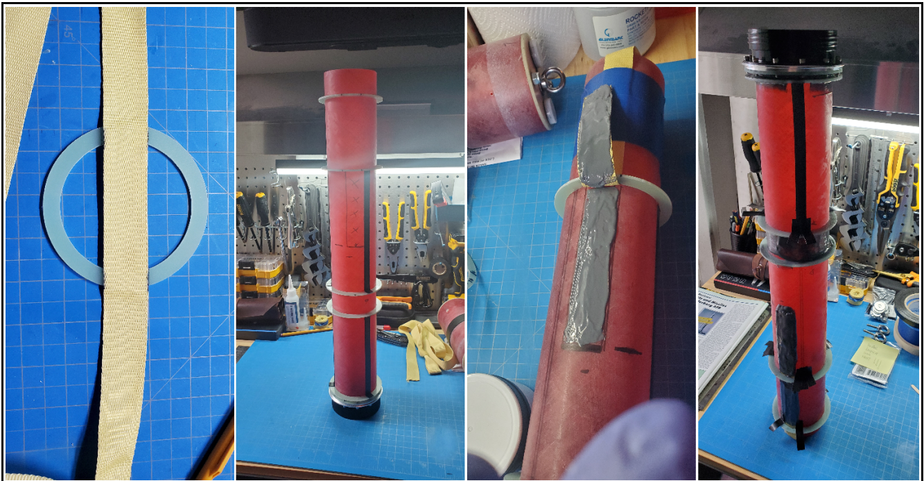
Fig. 14 – Left to right (Centering ring prep, centering ring mounting, y-harness threading and mounting, centering ring fillets laid down)
