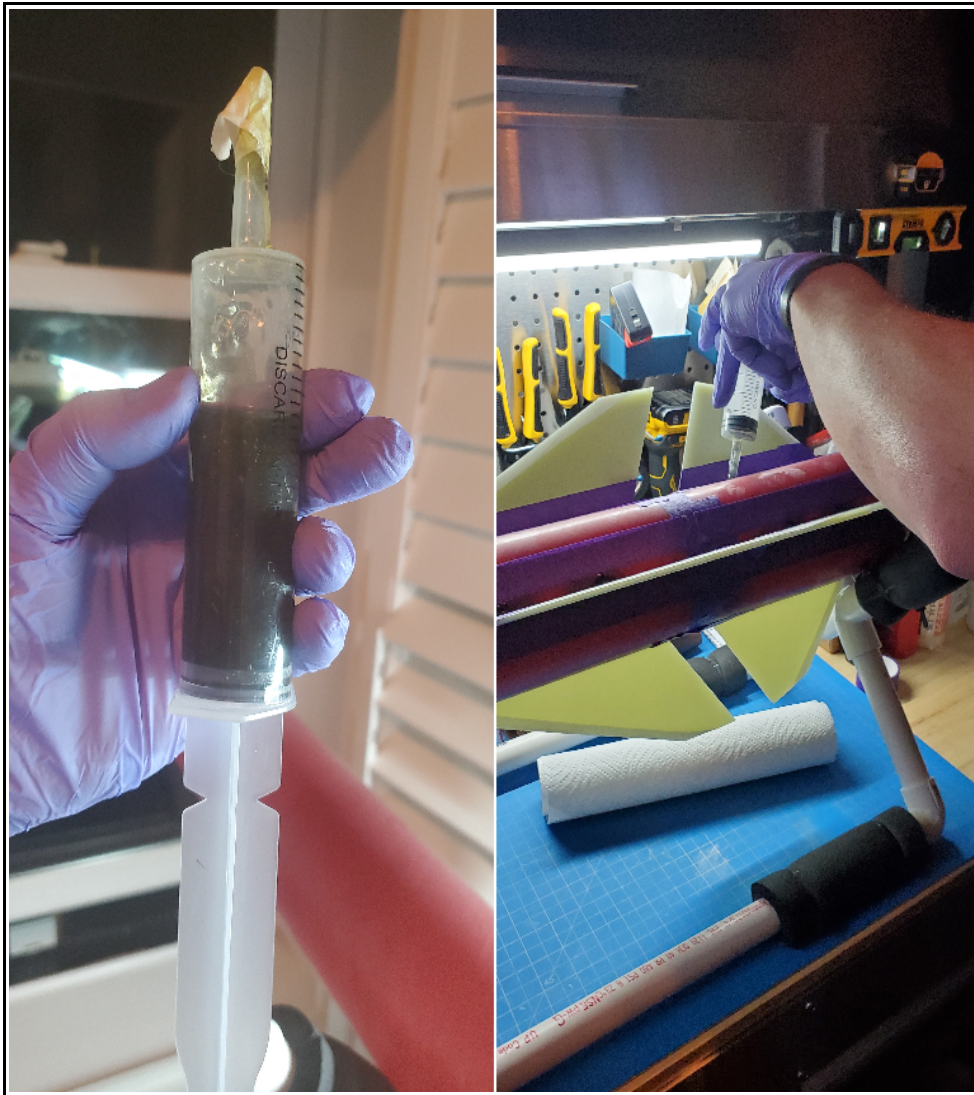
Fig. 17 – West 105 mixed w cut carbon fiber, internal fillet injection (5ml/slot)
