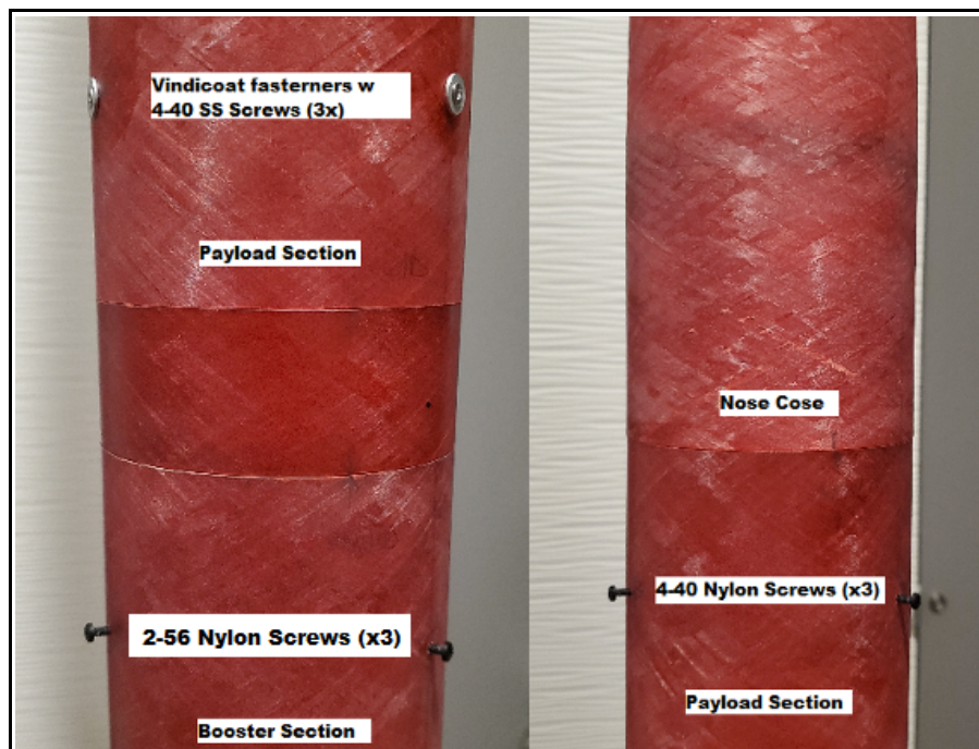
Fig. 22 – Nylon screws and Vindicoat Fasteners
