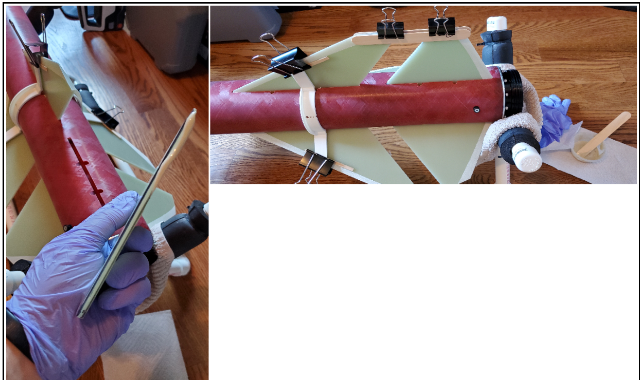
Fig. 16 – Root edge glue-up, fin alignment
