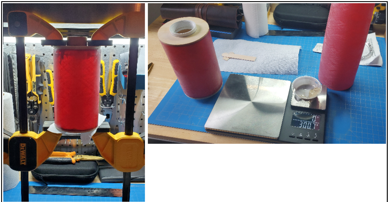
Fig. 21 – Nose cone bay sub-assembly glue up, nose cone mounting prep
