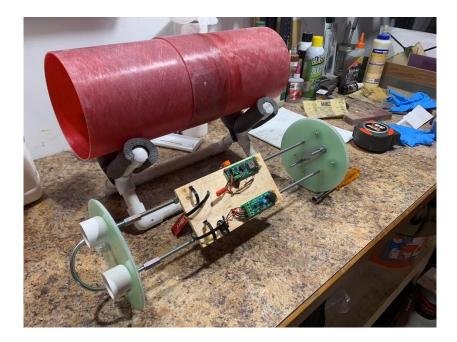
Also got the switch band epoxied into the center of the coupler.
