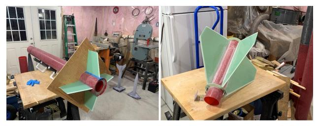
Weapons of choice here. The popsicle stick mixer is key. Each pair of fins needs about a full pump which is around 25 grams of resin. Noting quantities for my future self when I'm doing the next big rocket. Taped things off because I'm not a savage. Also note I taped over the Aeropack mounting holes so they weren't filled in accidently.
