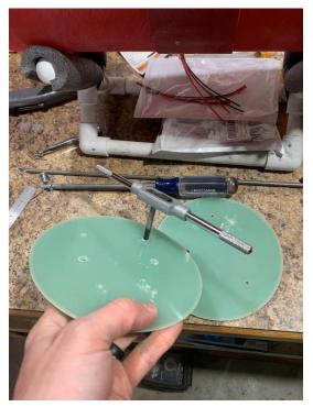
For this rocket I'm going to have the U-bolt for the drogue side attached directly to the two all thread going through the AV bay. This way the highest deployment forces aren't transferred into the rear bulkhead. Yes they'll in theory be applied to the front bulkhead, but that will be a force pulling it against the AV bay coupler, much more evenly distributed around the circumference, and shared with the hardware holding the payload section to the AV bay.
