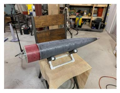
The weakest component here hardware wise is the 1/4-20 rod, and that's rated to 1,900 lb ultimate strength. This nose cone is about 5lb, so unless a 380G deployment event happens nothing should fail. Steady progress in the rocket lab.
