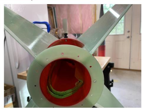
Got the fin can all the way in, tourniqueted the back of the airframe to clamp it around the aft centering ring, and epoxied the forward rail guide in with another weld nut.
