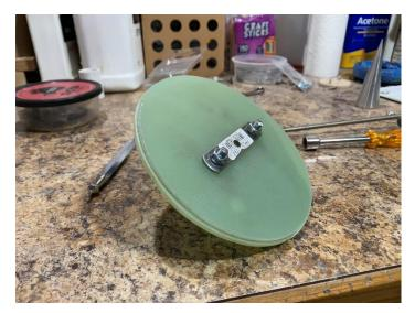
Here you can see the 1/4-20 rod double nutted and locktited. This is essentially the nose cone ready for paint! I'll drill shear pins last after running some calcs.
