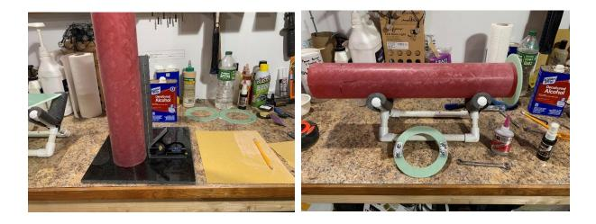
I tacked the centering rings in place with thick CA using the fins as spacers. **Make sure u-bolts and fins don't conflict!**
