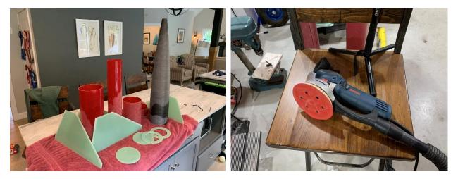
Nose cone construction started by bonding the shoulder. I decided I wanted this epoxied in place. I have done Wildman kits where you leave this loose and rely on threaded rod and a larger bulkhead to hold everything together, but I feel like that can distort the nose cone shape.
