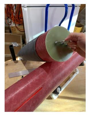
Then it was time to prepare and epoxy the fin can into the airframe. Before I slid this all the way in I epoxied in a weld nut for the aft rail guide. Notice how I taped all the kevlar harness up. This not only protects it from epoxy, but also any future ejection charges. Getting epoxy on the harness will concentrate forces and could be reduce overall strength.
